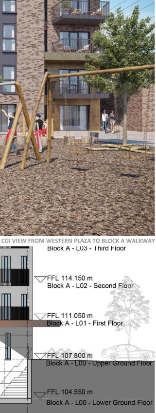
Detail Section thru Block A showing relationship of Block to Walkway
