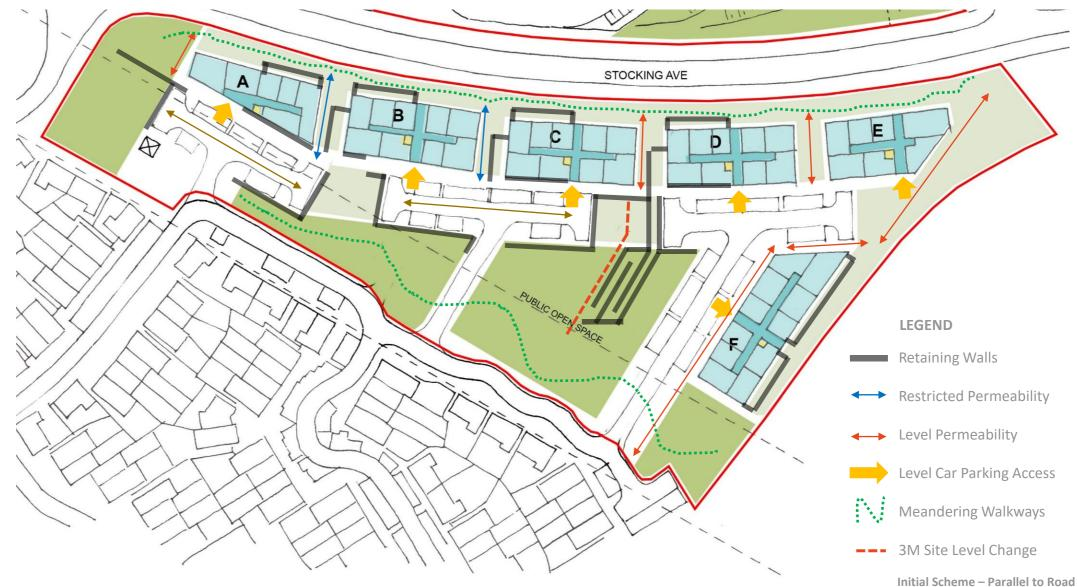
This block runs parallel with the north south site contours, thus allowing the perimeter of the block to be stepped following the contours rather than the entire block being either sunk or raised to address the contours.
